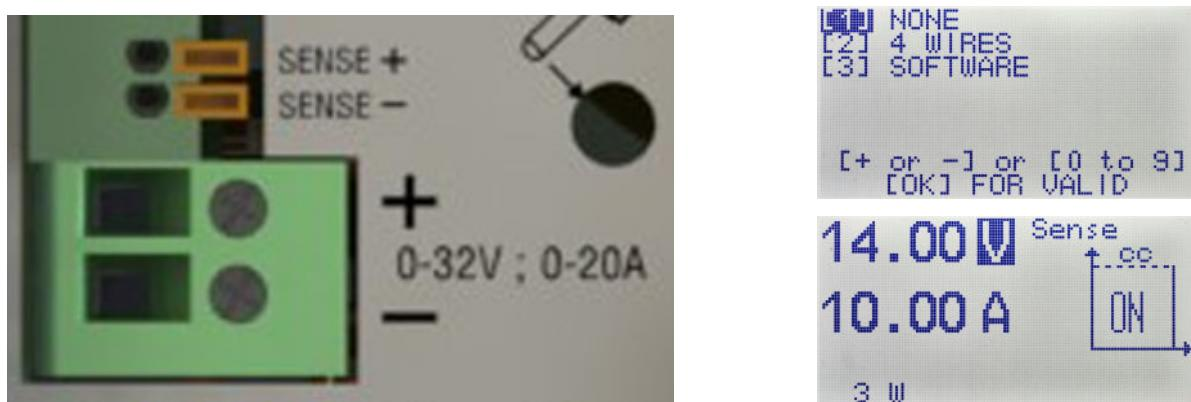
The "sense +" and "sense -" terminals must be connected to the + and - outputs as close as possible to the load. The recommended section of the conductors for power is 2.5 to 4mm<sup>2</sup> and 0.22 mm<sup>2</sup> minimum for the "SENSE"
