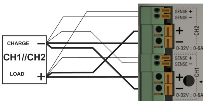
Tracking mode coupling (symetric)
