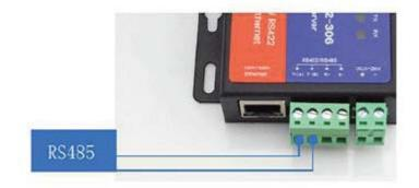
Connect with twisted wire (not supplied) T+ and T- to D+ et D- to ELC product (ALR3220, 3206D, 3206T,...).
